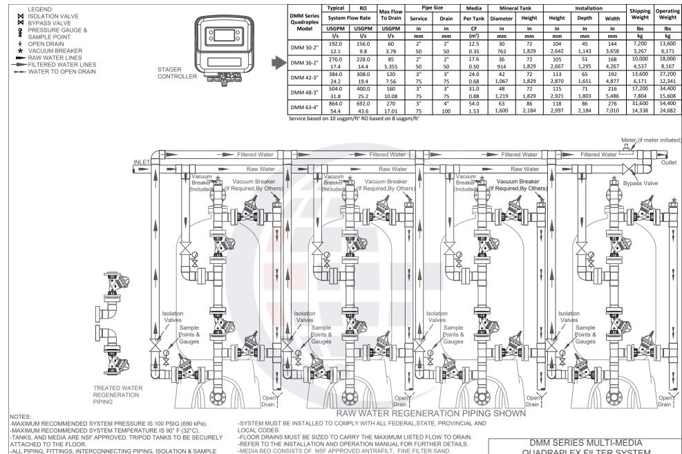
VALVES AND GAUGES SHOWN BY BROKEN LINES ARE BY OTHERS -SUPPLIED MANIFOLD IS SCH 80 PVC AND IS SUPPLIED WITH ONE VACUUM BREAKER. RECOMMENDED AIR RELEASE VALVE IS BY OTHERS. SYSTEM CAN BE PIPED AS RAW WATER OR TREATED WATER REGENERATION. -ALL PIPING MUST BE PROPERLY SUPPORTED AND BRACE TO HANDLE THE THRUST OF THE CHANGE OF WATER FLOW (BY OTHERS) -GLASS FIBER REINFORCED THERMOPLASTIC DIAPHRAGM VALVES ARE
